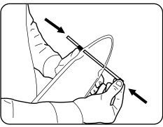
3. Place 1 off spacer on either end of the axle rod.
