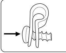
5. Place 2 off screws (removed from aperture) through the 2 off axles clamps.
