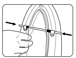
6. Place axle clamps over both ends of the axle rod.
