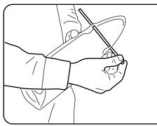
2. Place axle rod through holes in general waste flap.
