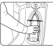
4. From the inside of the lid, line up the flap with the aperture so that the axle sits above the bosses.
